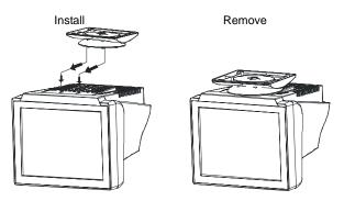
Figure 1. Installation and Removing of Pedestal
